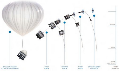
Scheme of the ascent profile for the Bloostar system. [Zero 2 Infinity]
