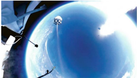
Left, Bloostar ignites at 25 km, before flying away (below). [Zero 2 Infinity]
